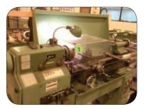
1 Rotating part of milling machine is fully guarded to prevent hand and finger injuries
