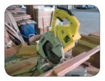
Defective guard must be repaired or replaced
