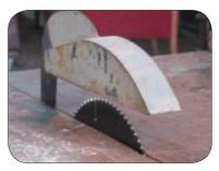
Saw guard must be adjusted as close to the timber piece as possible before cutting operation
