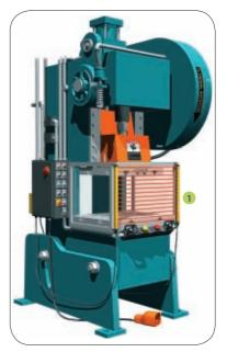
1 Part Revolution Power Press equipped with a safety light curtain, fixed enclosure guard, two-hands activation control and an emergency stop. (Picture courtesy of Omron STI)
