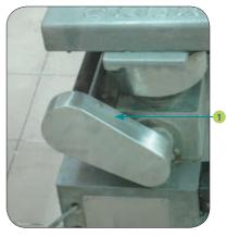
1 In-running nip of belt and pulley is fully enclosed to prevent hand and finger injuries
