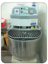
1 Flour mixer installed with interlocked guard
