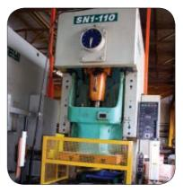
Light curtain not properly positioned to prevent operator's hands and fingers from straying into danger zone of the hydraulic power press
